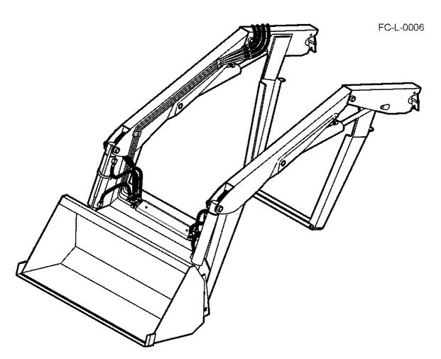
The Bush Hog 2297 Loader is designed for four-wheel drive tractors. They are intended to lift only loose materials that will fit in the bucket. All cylinders are double-acting. Parking stands support loader so tractor can be "driven in" for quick attaching.
